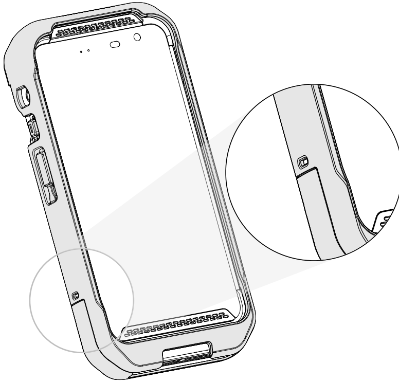
Figure 101 Attaching rugged boot_3
